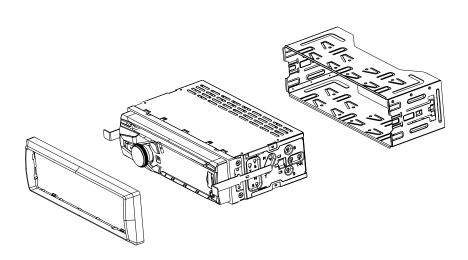
TYPICAL FRONT-LOAD DIN MOUNTING METHOD
